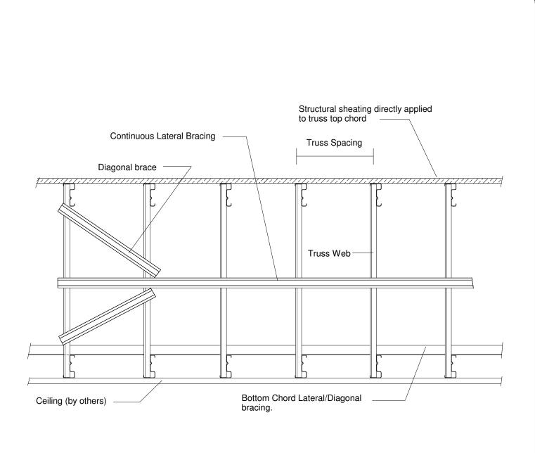
Bracing members typically attached with (2) #10 sds
